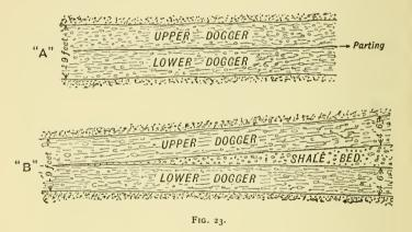
Our output of ore was at that time about 7,000 tons per week, nearly all of which was calcined in large kilns, in order to drive off the moisture and carbonic acid gas—a process which saved some 25 per cent. in railway freights. But unfortunately a few years later a change in the character of the seam developed which can best be explained by a rough sketch ; and in November 1882, after a long struggle for seventeen years, the work was brought to a standstill with a total loss of  $f_{150,000}$ .
